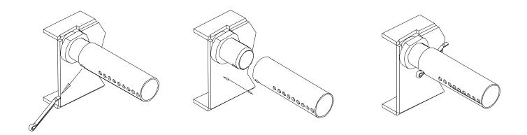
Figure 4.5 – Secondary air tube replacement
