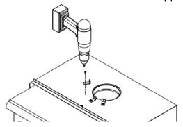
B) You can get from your dealer a liner fixation system (AC02006), sold separately. Follow the installation instructions provided with the liner fixation system.
