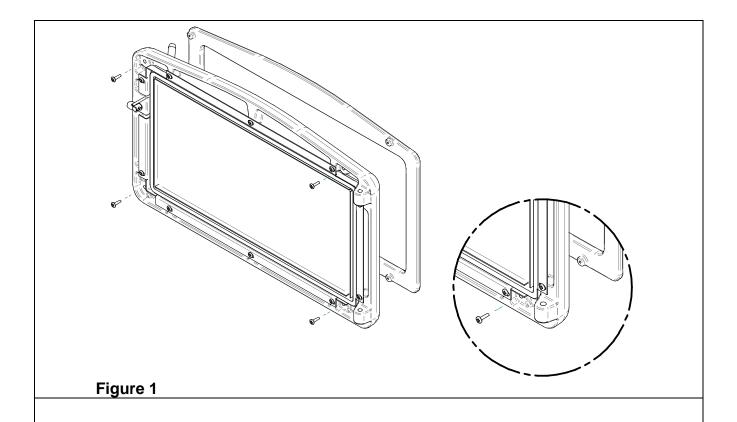
1- Position the overlay on the door frame and fix it in place from behind using the 4 screws.
