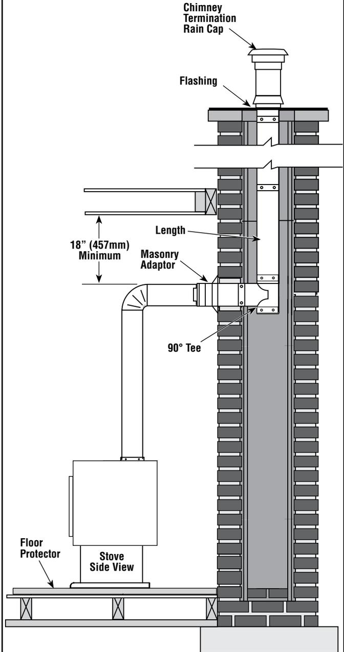
**Figure 6 - Connected to a Masonry Chimney**
