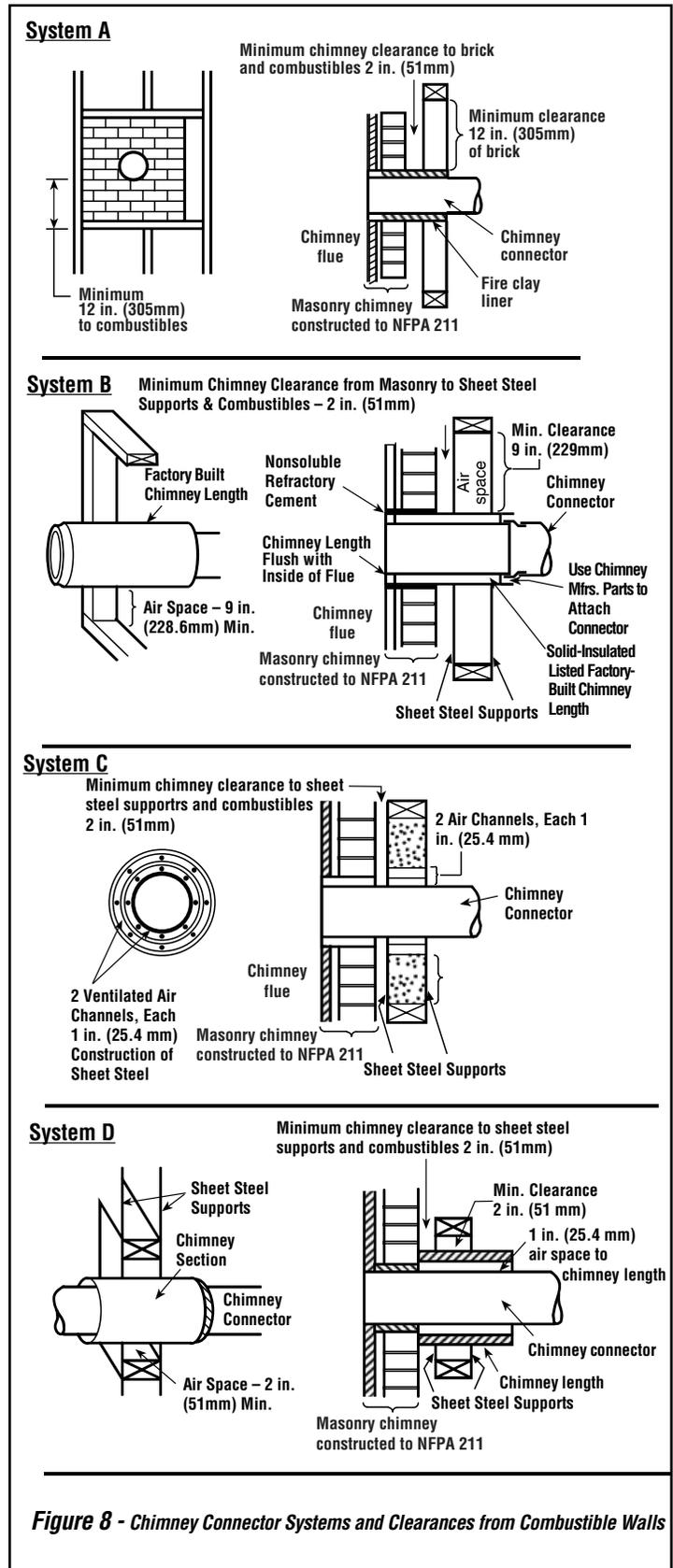
**Figure 8 - Chimney Connector Systems and Clearances from Combustible Walls**
