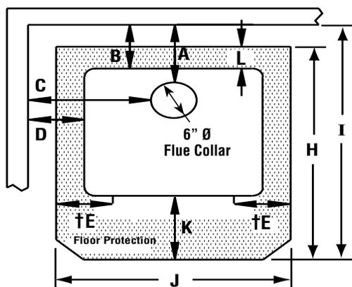
**Figure 3** Side View-Alcove & Parallel Installation
