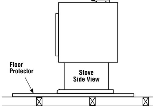
**Figure 5 - Typical Installation**
