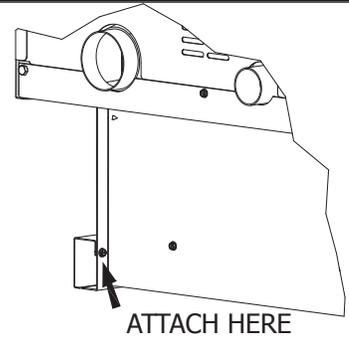
After trim assembly, attach to the pedestal base at the location shown using the screws provided.
