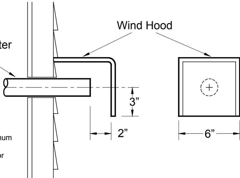
3. Only noncombustible pipe 2 inches (or greater) in diameter is approved to use for outside air connections (straight or flexible). PVC pipe is NOT approved and should NEVER be used.
