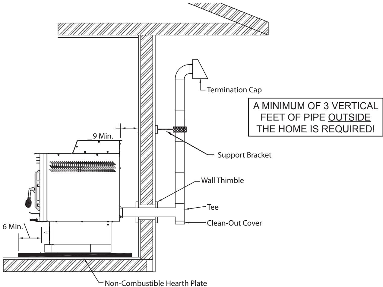
The Hearth Pad is not required under the unit if the floor is noncombustible but is required 6 inches (152mm) beyond the front of the unit and 6 inches (152mm) beyond each side of the door if the floor is a combustible floor. (wood flooring, carpet, linoleum, etc.)
