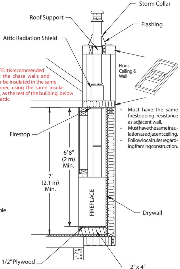
**NOTE:** It is recommended that the chase walls and floor be insulated in the same manner, using the same insulation, as the rest of the building, below the attic.
