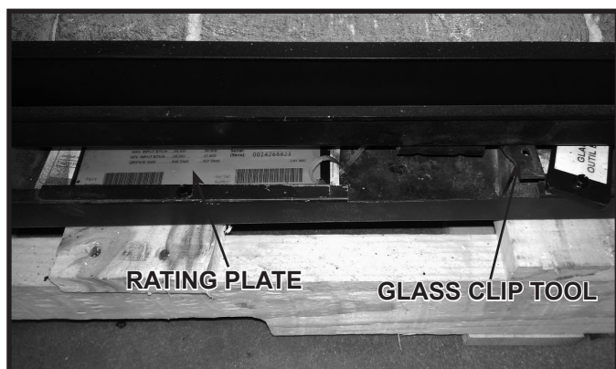
Figure 3.3 Rating Plate/Glass Clip Tool Location
