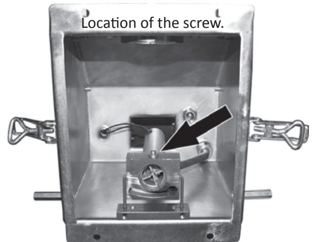
3. Use a screwdriver to lock the endstop into place.
