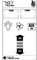
Figure 63 row buttons can also turn on or turn off the fireplace.
