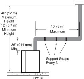
Figure 24 -Support Straps for Horizontal Runs
