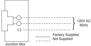
Figure 38 - Junction Box Wiring Diagram
