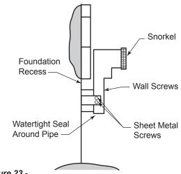
Figure 23 -Snorkel Installation, Recessed Foundation
