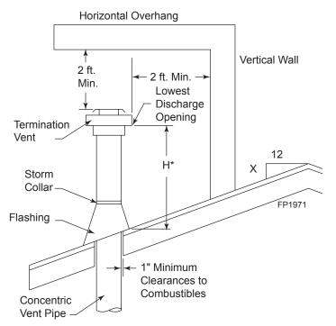
Figure 29 -Minimum Chimney Clearance
