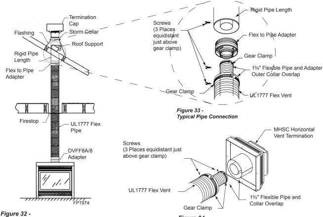
Figure 32 -Typical Vertical Flex Vent Installation
