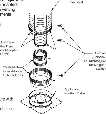
Figure 30 -Typical Appliance Connection
