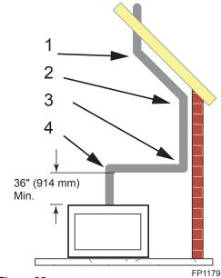
Figure 25 -Maximum Elbow Usage
