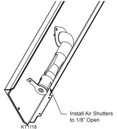
Figure 76 -Install Air Shutters -Conversion to Natural Gas
