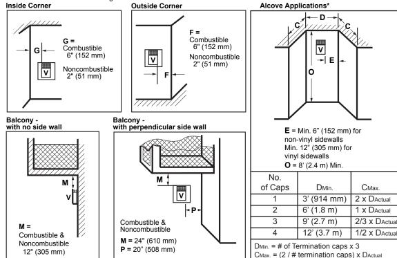
\*NOTE: Termination in an alcove space (spaces open only on one side and with an overhang) is permitted with the dimensions specified for vinyl or non-vinyl siding and soffits. 1. There must be a 3' (914 mm) minimum between termination caps. 2. All mechanical air intakes within 10' (1 m) of a termination cap must be a minimum of 3' (914 mm) below the termination cap. 3. All gravity air intakes within 3' (914 mm) of a termination cap must be a minimum of 1' (305 mm) below the termination cap.
