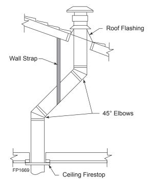
Figure 26 Offset with Wall Strap and 45° Elbows
