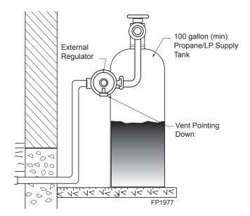
Figure 35 External Regulator with Vent Pointing Down
