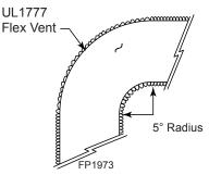
Figure 31 -Minimum Radius for Flex Vent Section
