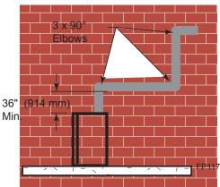
Figure 18 - Maximum Three (3) 90° Elbows Per Installation
