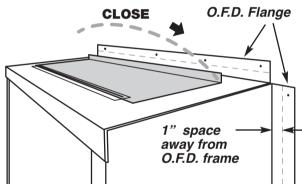
NOTE: **CLOSE** top vent door while loading furnace to keep smoke & gases out of greenhouse while loading furnace. Reopen top vent door before closing O.F.D.
