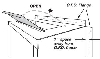
WARNING: Top vent door must be **OPEN** when O.F.D. is closed to allow air circulation around front of furnace.
