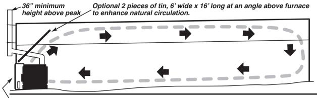
When possible, locate furnace on north or west end of greenhouse. Above drawing shown with outside fire door.
