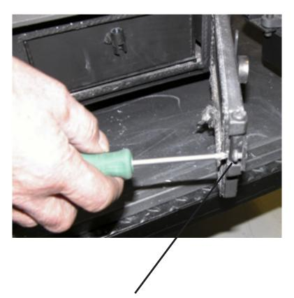
Adjust the screw at the end of the ash pan door lever to give a positive action when closing. Do not over adjust. The closing action of the lever should have a gentle resistance.
