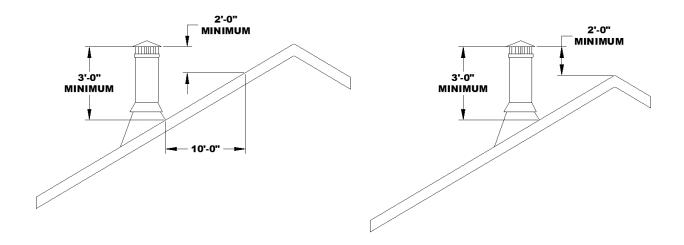
Figure 8 - Chimney Height Requirements
