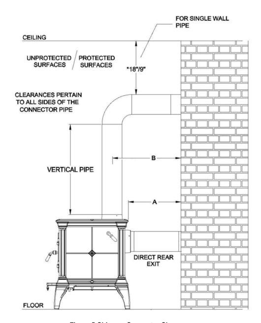
**Figure 5 Chimney Connector Clearances**
