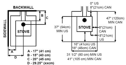
When installed on a combustible floor, non-combustible floor protection is required to cover the area beneath the heater, and extend at least 16"(41cm) [18" (46cm) CAN] to the front and 8"(21cm) beyond each side of the fuel loading and ash removal openings [side of stove in CAN], the floor protection must extend under the flue connector and extend 2" beyond each side of pipe.
