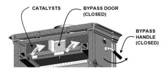
Figure 14 - Bypass Closed
