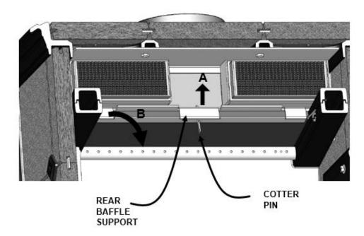
Figure 22 - Removing the Rear Baffle
