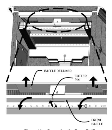
Figure 18 - Removing the Front Baffle
