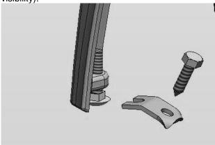
Figure 10 - Lock Down Detail
