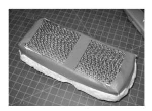
Figure 20 - Installing Gasket on Catalyst
