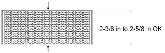
Figure 21 - Acceptable Catalytic Distortion
