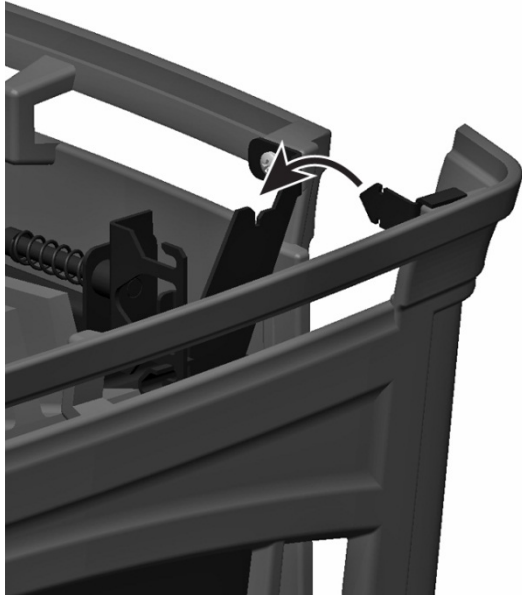
Figure 11 – Front Panel Mounting Tang Detail
