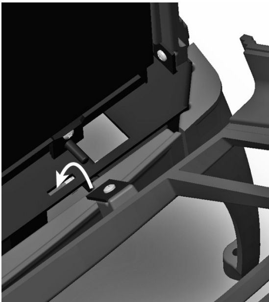
Figure 12 – Front Panel Retaining Slots
