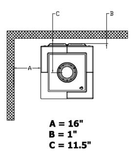
Caution: These clearances represent minimum distances in all cases, which, through testing in an independent laboratory to ANSI and CSA standards, will prevent fire or spontaneous combustion. We do not control the combustible materials exposed to heat by this product; therefore, an assessment must be made by the installer to prevent consequential damage of walls and flooring.
