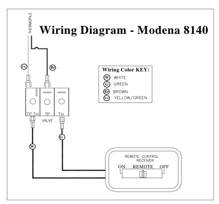
Figure 8: Modena 8140 Wiring Diagram
