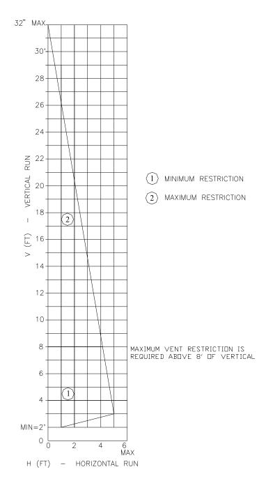
NO RESTRICTOR PLATE REQUIRED UNDER 5' VERTICAL
