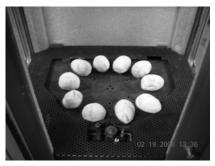
Install 10 stones in a circle pattern. The stones must not cover the burner ports of the outer ring on the burner, and should fit in between the burner ports.
