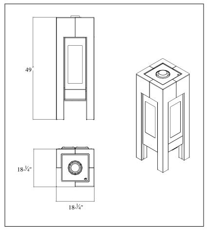
Figure 1: Modena DV Model 8140 Dimensions
