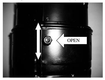
Figure 5: Restrictor in open position
