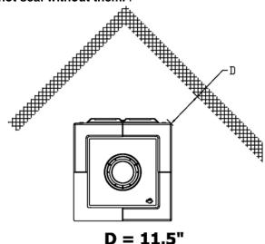
Figure 2 - Clearance to Combustibles
