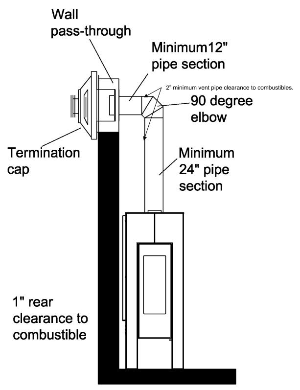
Figure 3: Minimum Vent Configuration and Clearances
