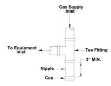
Figure 10: Typical Sediment Trap (required in all installations)
