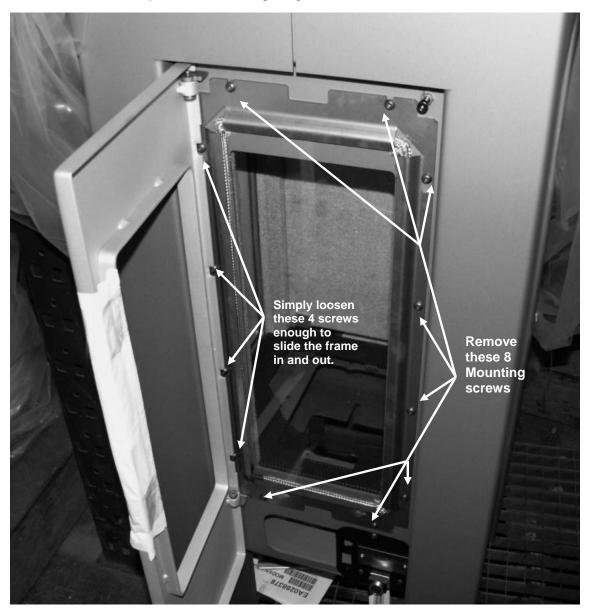
Figure 16: Glass frame mounting screws
