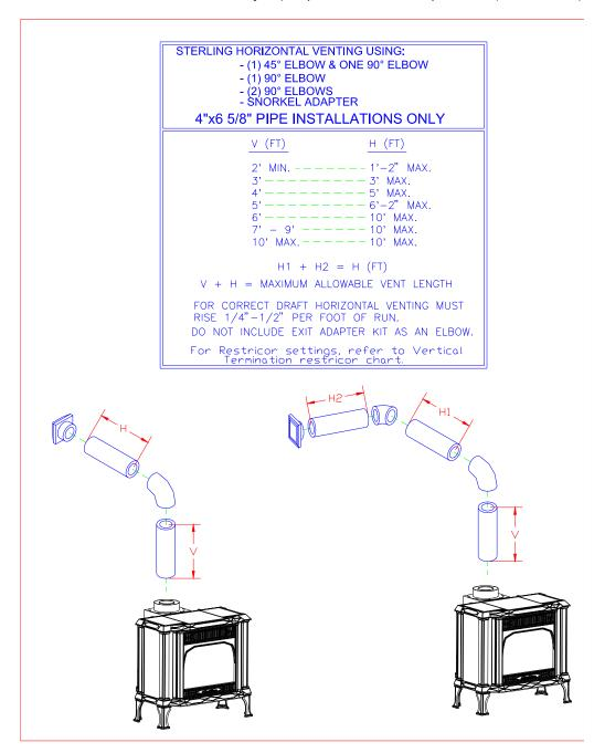
Note: All top exit configurations require a minimum of a 24" section of pipe directly off the unit.
