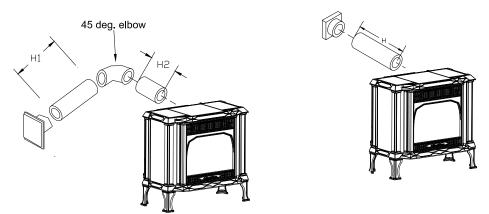
CENTERLINE OF PIPE IS 21.25" ABOVE THE FLOOR
