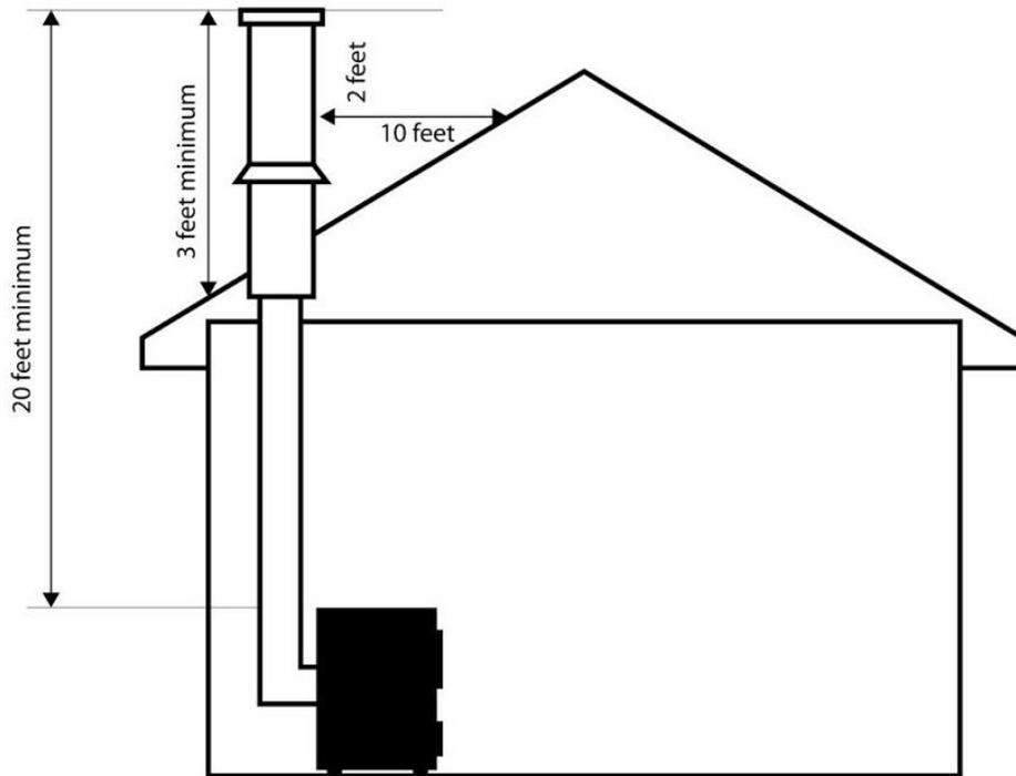
1. The cookstove must have its own chimney flue. One cookstove per flue.
