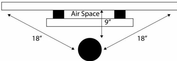
According to NFPA Standards, single-walled stove pipes can be within 9 inches of a combustible, provided an approved fire retardant material is utilized. It must also be covered with 28 gauge sheet metal and spaced out 1" on non-combustible spacers.
