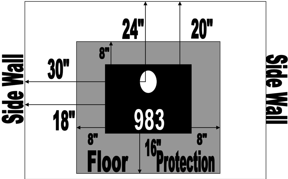
Free Standing Installation: Clearance to Combustible Material:
