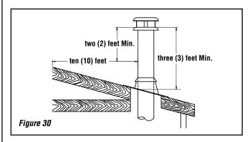
NOTE: 2" clearance to combustibles around chimney components required.
