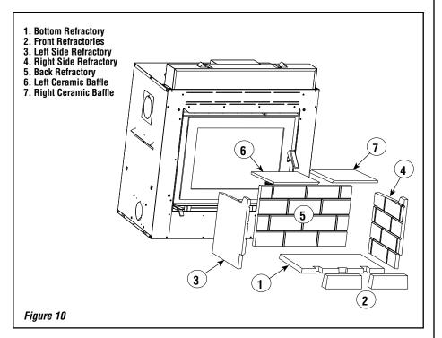
The intense heat of the fire will normally cause hairline cracks in the refractory. These cracks can be minimized by proper curing as described in "First Fires". They will not normally diminish the effectiveness of the refractory. If large cracks develop, then the refractory should be replaced. To replace the refractory bricks, follow these steps (see *Figure 10*):
