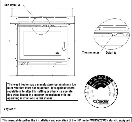
This manual describes the installation and operation of the IHP model WRT3920WS catalytic equipped wood heater. This heater meets the 2020 U.S. Environmental Protection Agency's certified to comply with 2020 particulate emission standards using crib wood. Under specific test conditions this heater has been shown to deliver heat at rates ranging from 10,900 to 35,600 Btu/hr.
