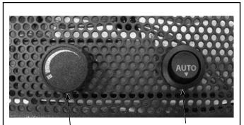
Blower Speed Control Knob (rheostat) Manual / Auto Rocker Switch
