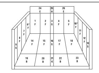
Firebox Brick Layout as Viewed from the Front \* Bricks 6 and 10 fit up against the back of the firebox.
