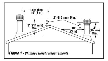
To pass inspection in nearly any jurisdiction, the chimney must meet both safety and exhaust flow requirements. The (3' by) 2' by 10' rule applies to both masonry and factory-built chimneys.
