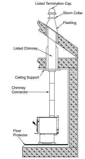
Figure 14.1 - Prefabricated Interior Chimney
