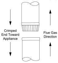
Secure pipe sections with a minimum of 3 screws
