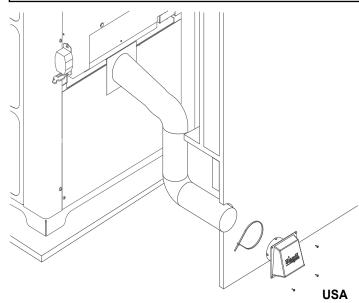
Figure 16.2 - Floor Installation
