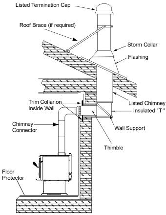
Figure 13.1 - Prefabricated Exterior Chimney
