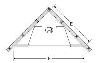
Note: If this is an outside corner, the minumum distance between the vent and the outside corner is 6" (15cm) with AstroCap termination cap or 12" (30cm) with Rigid Vent termination cap. (For example Dura-Vent)
