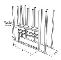
Note: Three horizontal steel studs must be installed after the unit is in position and the venting, gas and electrical is installed. The horizontal studs allow the non-combustible wall board to be attached and supported.
