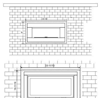
7. For material such as brick, stone, etc that extends less than 3-1/8", the minimum opening dimensions noted below must be adhered, when finishing around the faceplate. This is to ensure the removal of the faceplate and for the safe operation of this appliance.
