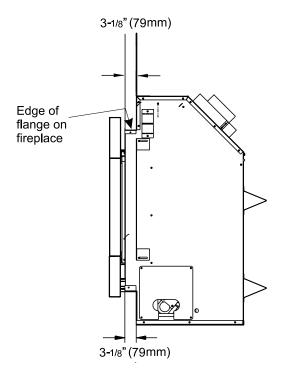
**Important:** 1/2" gap required between faceplate and finished wall when using part 4 pc. faceplate. When using the outer faceplate the 1/2" gap is not necessary.
