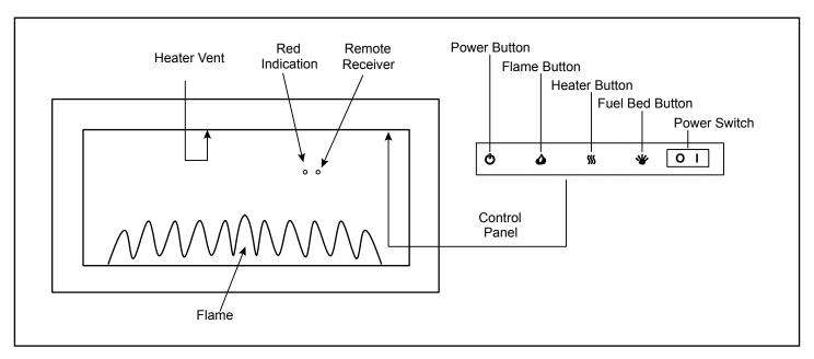
Figure 5.1 Manual Operating Switches and Indicator Lights
