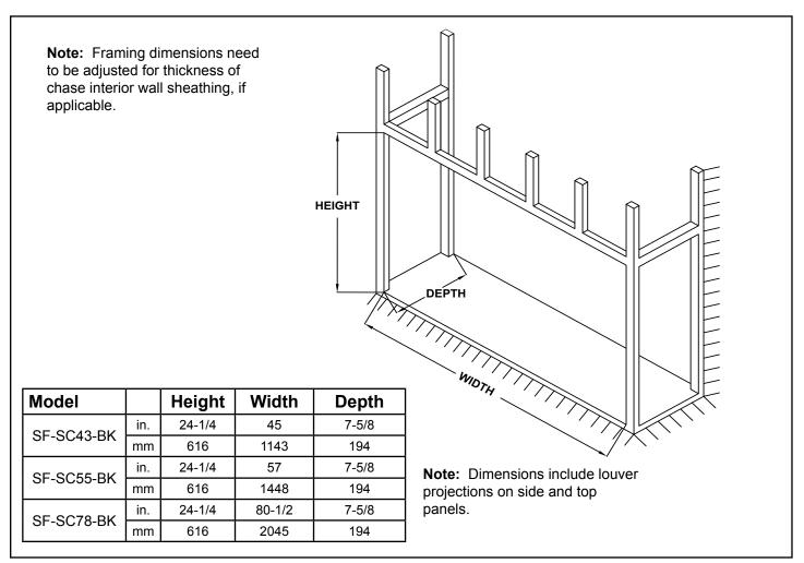
Figure 4.1 Framing Dimensions
