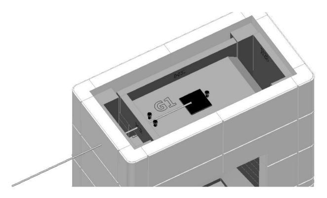
Install bypass trap according to the illustration
