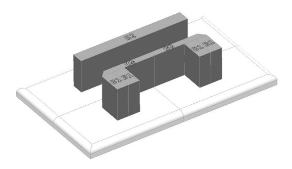
Line up the "B" parts according to the grooves on "A" parts.
