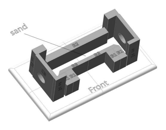
Add 1 1/2" thick of sand mixed with sodium silicate everywhere in the lower part of the channel \*See the "Important advice" page for the mixture (page 1)
