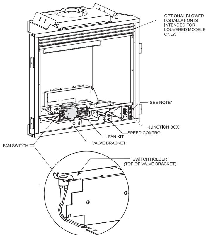
**\*NOTICE:** Refer to Junction Box wiring instructions on page 91 for proper operation.
