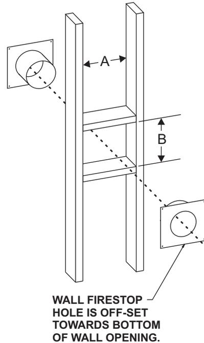
WALL FIRESTOP HOLE IS OFF-SET TOWARDS BOTTOM OF WALL OPENING.
