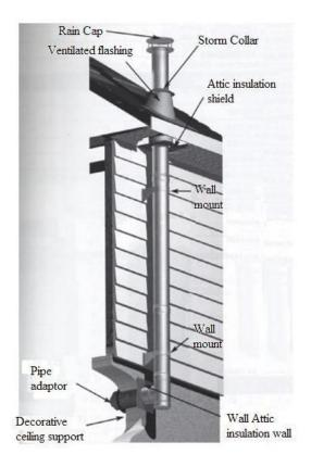
The *Tison* and *Cuisiniere model*) must be installed in accordance with the applicable local laws or the CAN/CSA - B365 ULC S635, ULC S640 standards. For the chimney, follow the chimney manufacturer's instructions.
